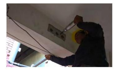
Figure 17: Photograph showing Schmidt Hammer Test
