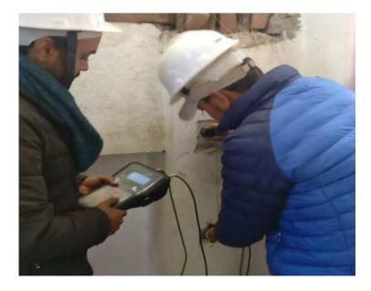
Figure 18: Photograph showing Schmidt Hammer Test
