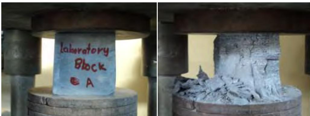
Figure 15: Photograph showing Compressive Strength Test of Stone
