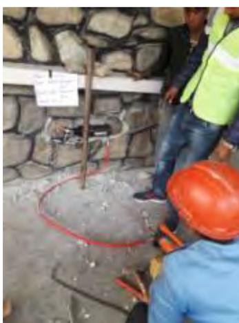
Figure 14: Photograph showing Bed Joint Shear Test
